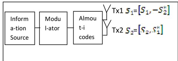
Fig.4 A block diagram of the Alamouti space-time encoder.
