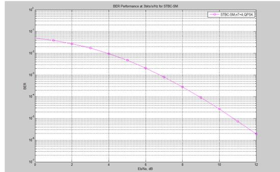
Fig.9 BER performance of STBC SM system under QPSK modulation for 4 transmitting antennas
