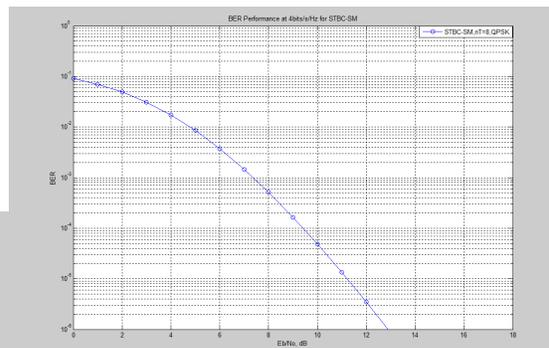
Fig.11 BER performance of STBC SM system under QPSK modulation for 8 transmitting antennas.
