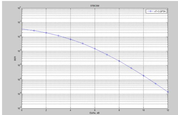
Fig.6 BER performance of QPSK modulation for 3 transmitting antennas
