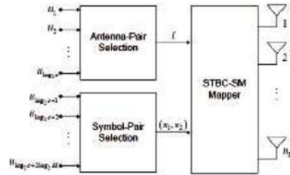
Fig.3. The block diagram of the STBC-SM transmitter
