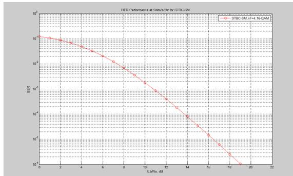
Fig.12 BER performance of STBC SM system under 16-QAM modulation for 4 transmitting antennas
