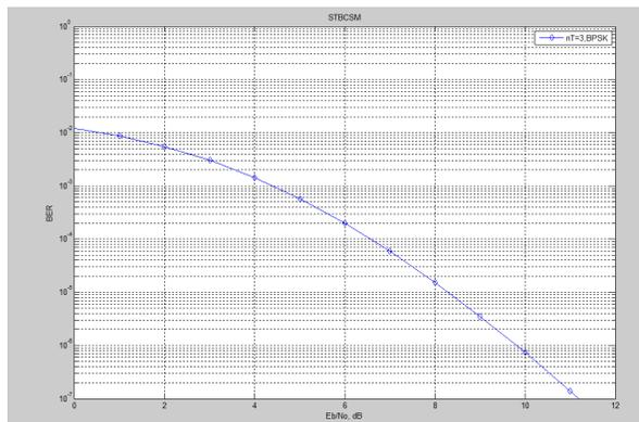
Fig.7 BER performance of BPSK modulation for 3 transmitting antennas
