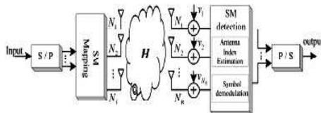
Fig.5 SM system diagram
