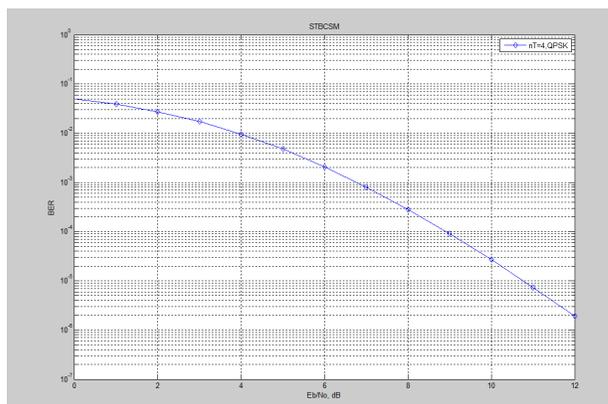
Fig.8 BER performance of QPSK modulation for 4 transmitting antennas
