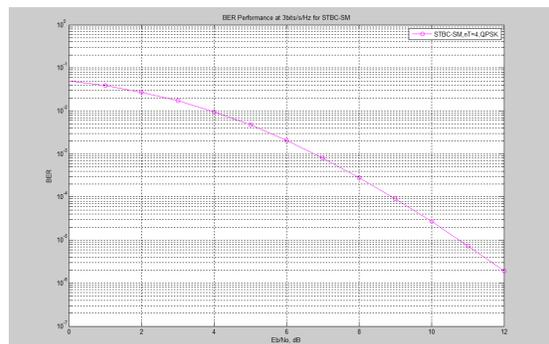
Fig.10 BER performance of STBC SM system under QPSK modulation for 4 transmitting antennas
