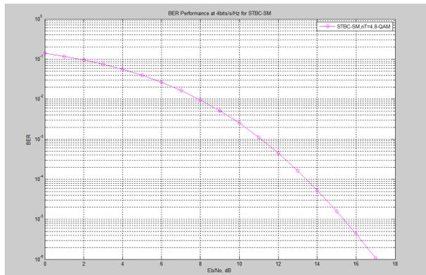
Fig.13 BER performance of STBC SM system under QAM modulation for 4 transmitting antennas
